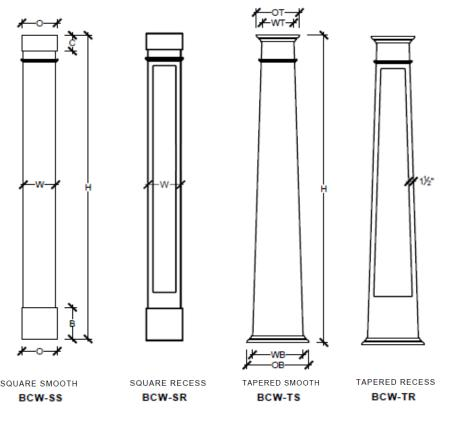
Spectis Box Column Wraps are made with 1/2" material that is weather and insect proof and is maintenance-free. They can be used as exterior or interior columns as they will not rot or twist. The recess in the Square and Tapered Recess columns is 1/2" deep.
