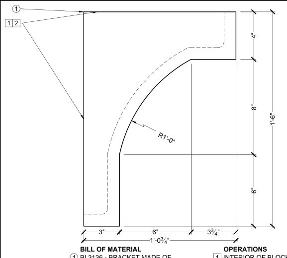
1 BL3136 - BRACKET MADE OF POLYURETHANE
