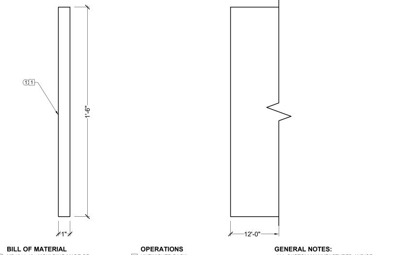
① MD1011-18 - MOULDING MADE OF POLYURETHANE.
