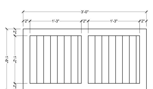
1 SHL-2-1836 SHUTTER MADE OF POLYURETHANE AND/OR PVC
